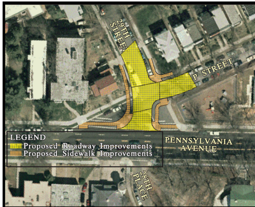
FIGURE 39: The realignment of Pennsylvania Avenue, SE/29 th Street/28 th Place
