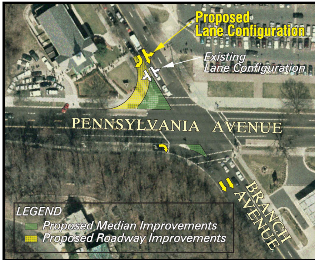
FIGURE 42: Establish an eastbound free flowing right turn onto southbound Branch Avenue.
