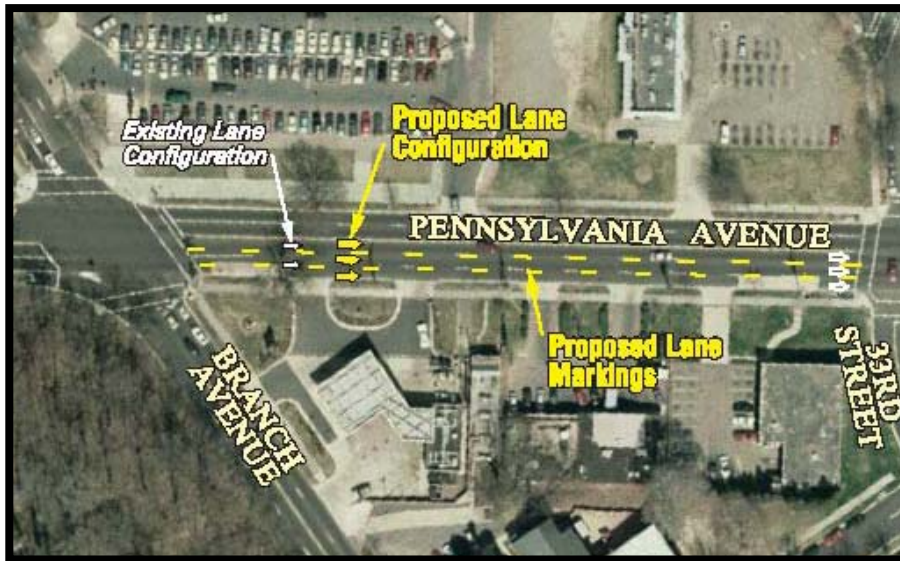
FIGURE 36: Eastbound Transition at Branch Avenue
