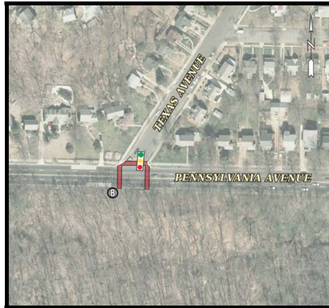
FIGURE 26: Proposed traffic signal and pedestrian improvements at Pennsylvania Avenue, SE/Texas Avenue.
