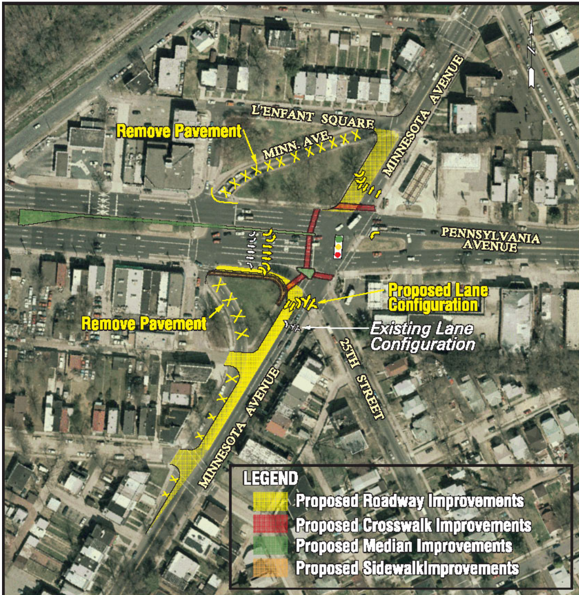
FIGURE 37: Reconfiguration of Pennsylvania Avenue, SE/Minnesota Avenue/25 th Street Intersection
