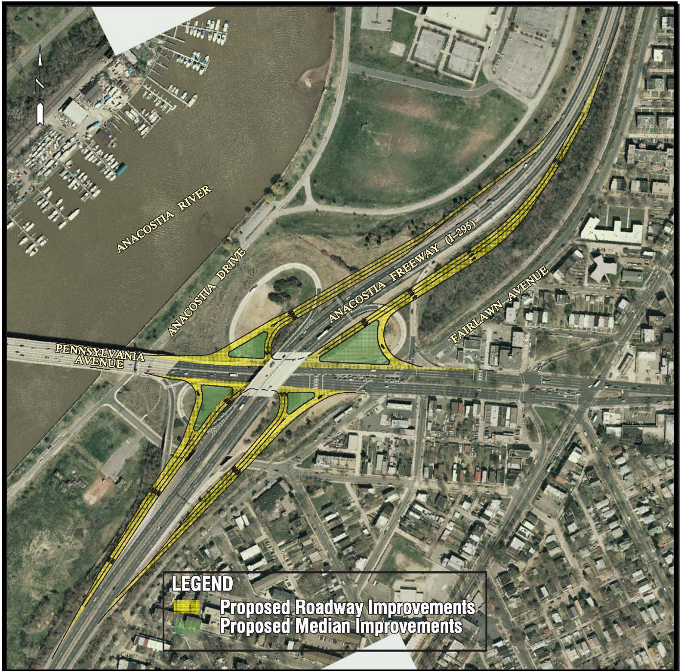
FIGURE 41: Single Point Urban Diamond interchange at Anacostia Freeway (I-295)/Pennsylvania Avenue, SE
